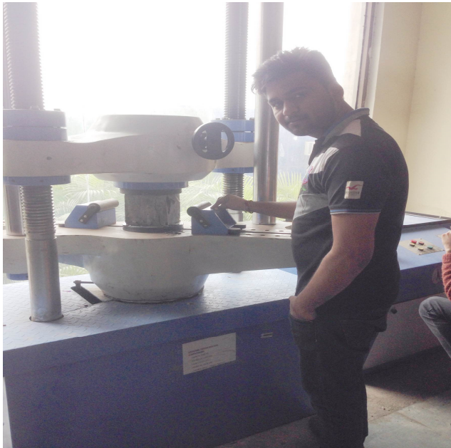
Figure 3 Testing of concrete on UTM.
